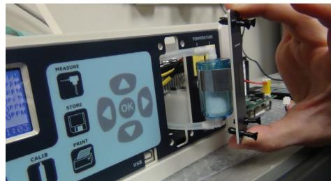
The condensation filter is typically replaced much less frequently than the line filter and should be replaced if it becomes saturated with water. This filter is accessed by opening up the analyzer. More details can be found in the Maintenance section (Chapter 12) of the complete Si-CA 8500 user manual.
